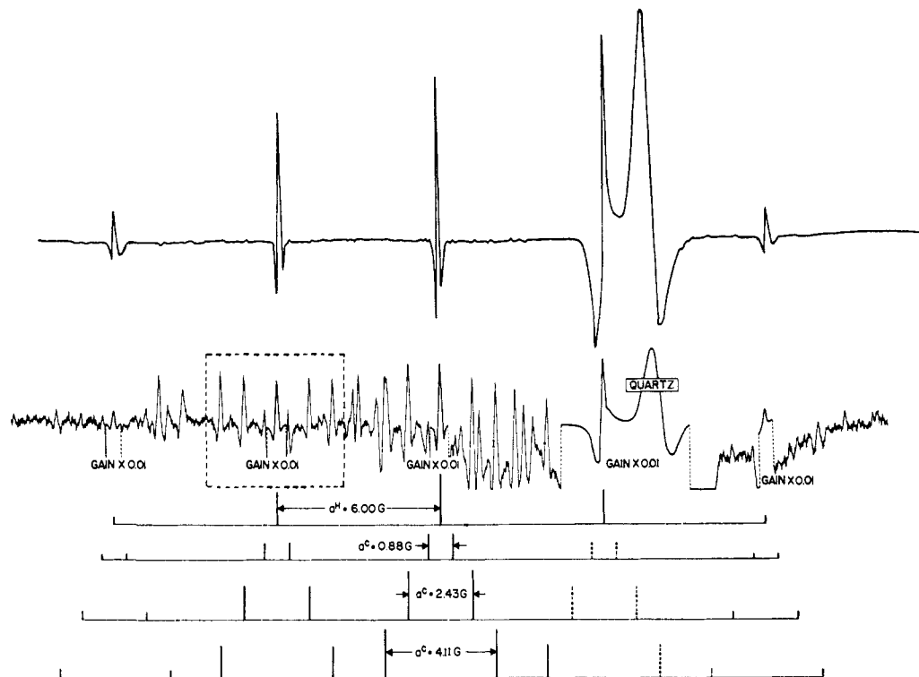
Figure 5. The esr spectrum of the radical present during the irradiation of a 10^{-3} M solution of reductic acid. A very intense 6.00 G quintet of radical II is present. At a 100-fold higher gain a considerable number of additional lines are apparent. The only lines present that can be appropriately assigned to ^{13}C -containing radicals are at the positions indicated by the three lowermost stick spectra. The three pairs of lines of relative intensities 0.01, 0.01, and 0.005 are readily seen in the enclosed area around the second line of the main spectrum.
